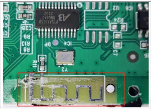
The antenna is PCB antenna.
