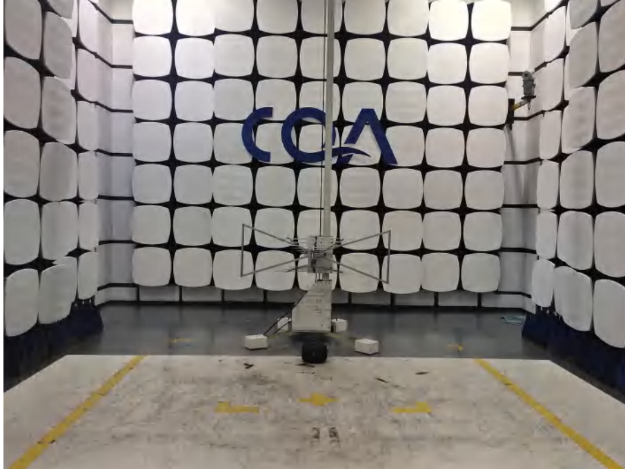
Radiated emission Test Setup (30MHz~1GHz)
