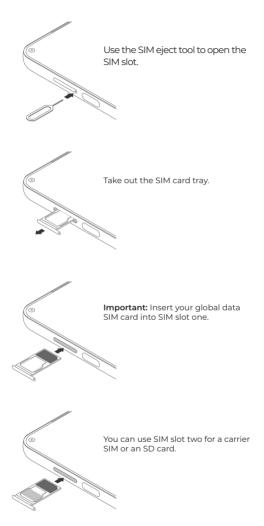
Insert the SIM tray back into the device.
