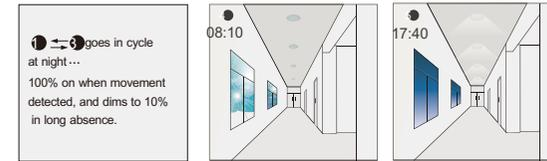
At night... goes in cycle at night... 100% on when movement detected, and dims to 10% in long absence.
