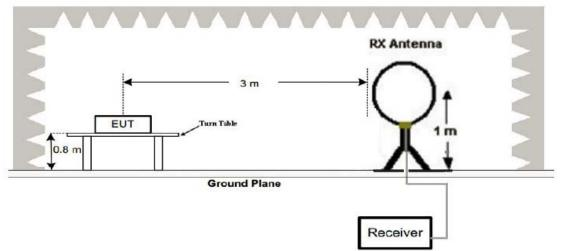
(2) Radiated Emission Test-Up Frequency 30MHz~1GHz
