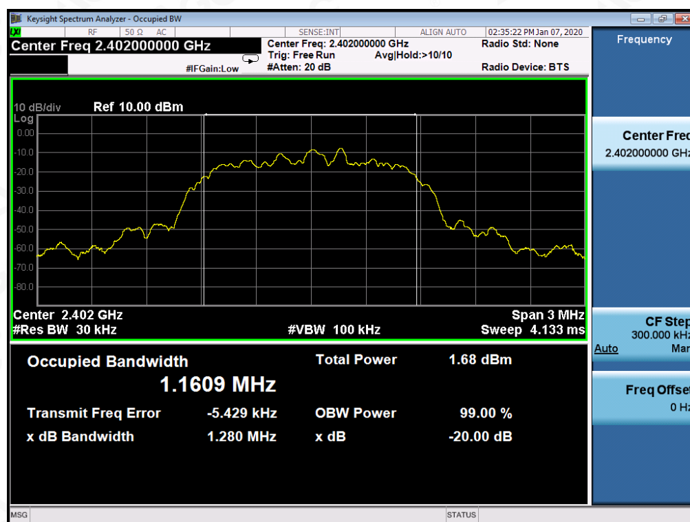
TEST PLOT OF BANDWIDTH FOR LOW CHANNEL
