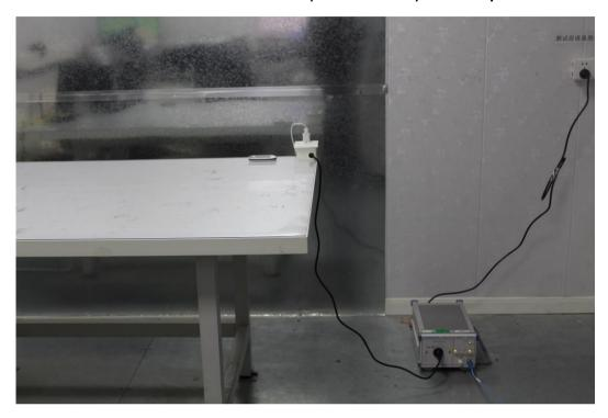
**Radiated Emissions Test Setup**
