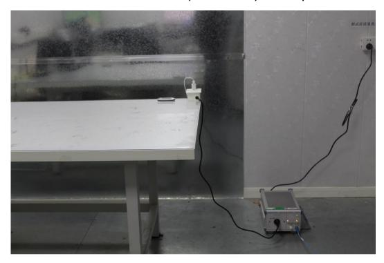
**Radiated Emissions Test Setup**
