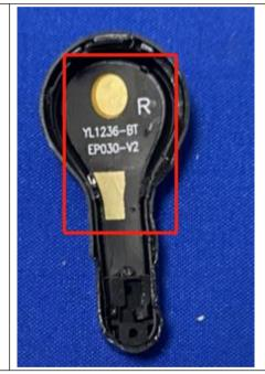
The antenna is FPC antenna. The best case gain of the antenna is -1.5 dBi.
