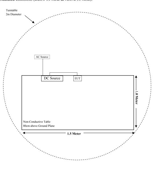
For Radiated Emissions (Below 30 MHz & Above 30 MHz):
