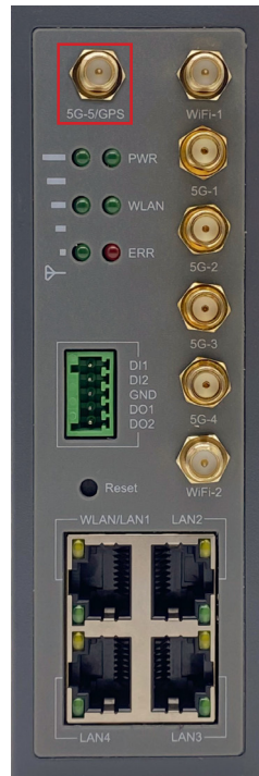
Figure 24. GPS Antenna Connectors (GPS Version)
