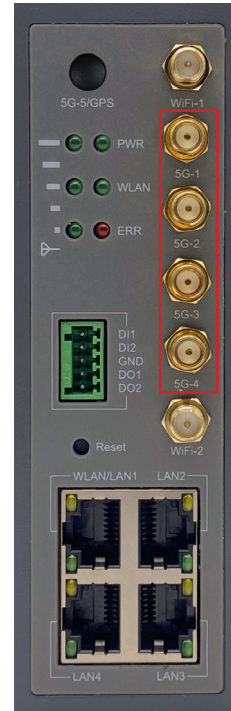
Figure 23. Cellular Antenna Connectors (non-GPS version)
