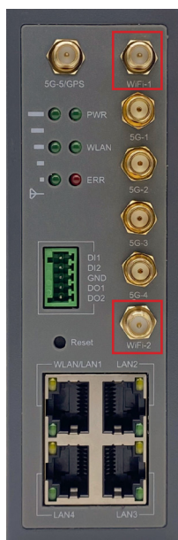
Figure 25. WiFi Antenna Connectors (GPS Version)
