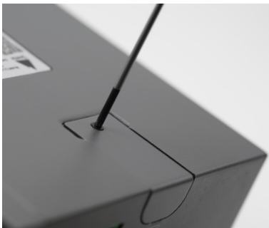
Figure 19. Remove SIM cover plate
