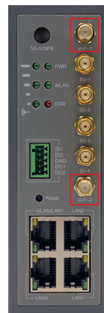
Figure 26. WiFi Antenna Connectors (non-GPS version)
