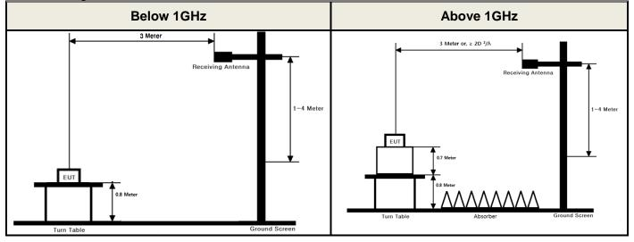
These measurements were performed at 3 test site. The equipment under test is placed on a non-conductive table 1.5meters above a turntable which is flush with the ground plane and 3 meters (for below 1GHz: 0.8-m) from the receive antenna. For measurements above 1GHz absorbers are placed on the floor between the turn table and the antenna mast in such a way so as to maximize the reduction of reflections. For measurements below 1 GHz, the absorbers are removed.
