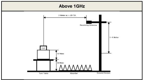
These measurements were performed at 3 m test site. The equipment under test is placed on a non-conductive table 1.5-meters above a turntable which is flush with the ground plane and 3 meters from the receive antenna. For measurements above 1GHz absorbers are placed on the floor between the turn table and the antenna mast in such a way so as to maximize the reduction of reflections. For measurements below 1 GHz, the absorbers are removed.
