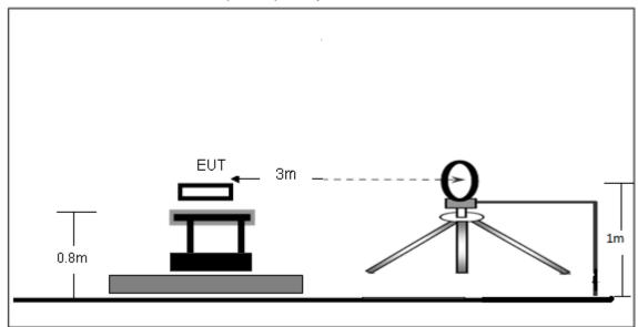
(B) Radiated Emission Test-Up Frequency 30MHz~1GHz
