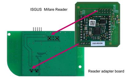
Installation and integration of reader adapter board into IT 82xx (Fig. IT 8210):
