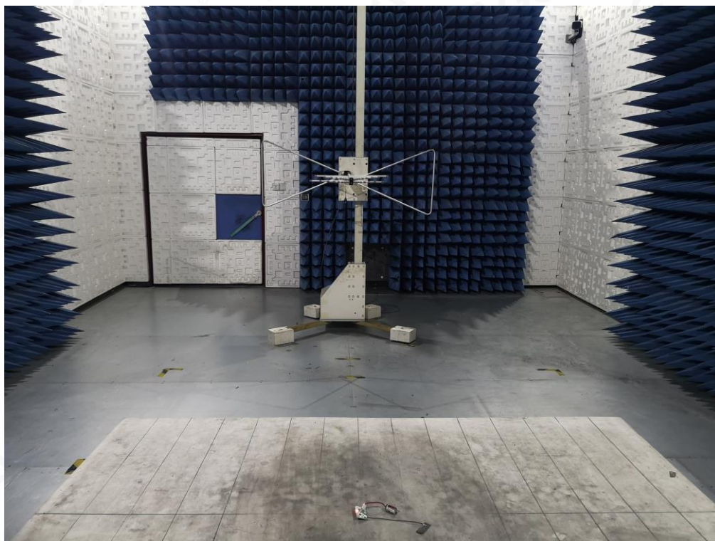
FCC RADIATED EMISSION TEST SETUP ABOVE 1GHZ
