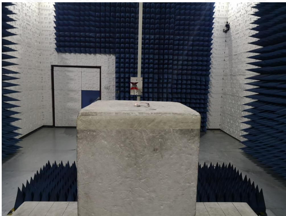
FCC RADIATED EMISSION TEST SETUP ABOVE 1GHZ
