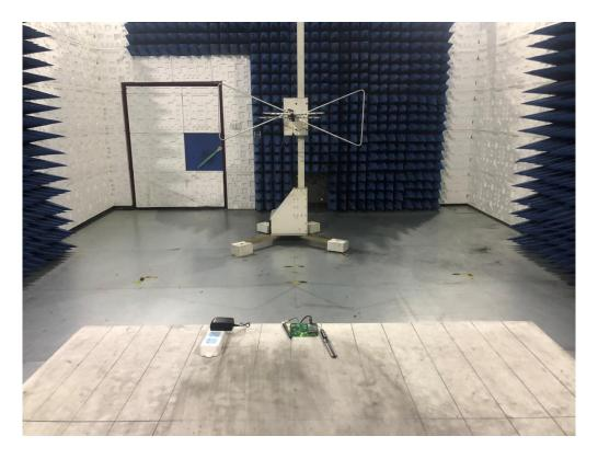
FCC RADIATED EMISSION TEST SETUP ABOVE 1GHZ
