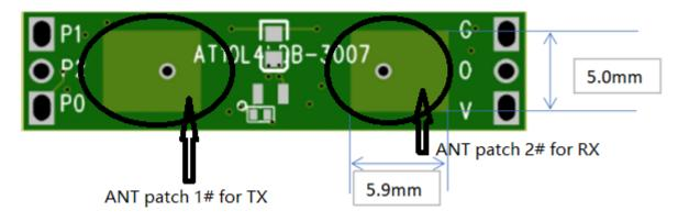
ANT patch 1# and ANT patch 2#, having the same size, make up the antenna system of EUT. Refer to above table and picture for the dimensions of antenna of EUT.
