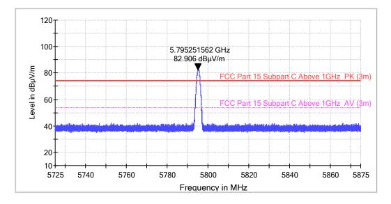
Remark: The PK values of the frequency of 5725MHz and 5875MHz are below 54dB  $\mu$  V/m. Horizontal
