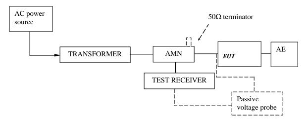
Test Setup and Procedure:
