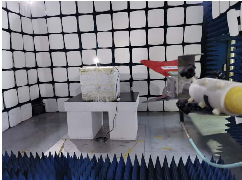
Radiation Emission Test Setup (1GHz to 18GHz)
