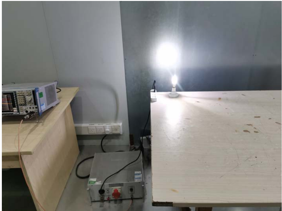
Conducted Emission Test Setup
