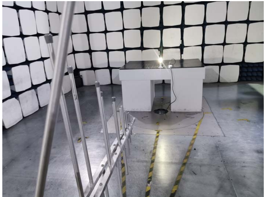
Radiation Emission Test Setup (30MHz to 1GHz)
