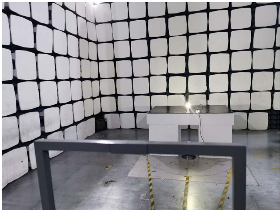
Radiation Emission Test Setup (Below 30MHz)
