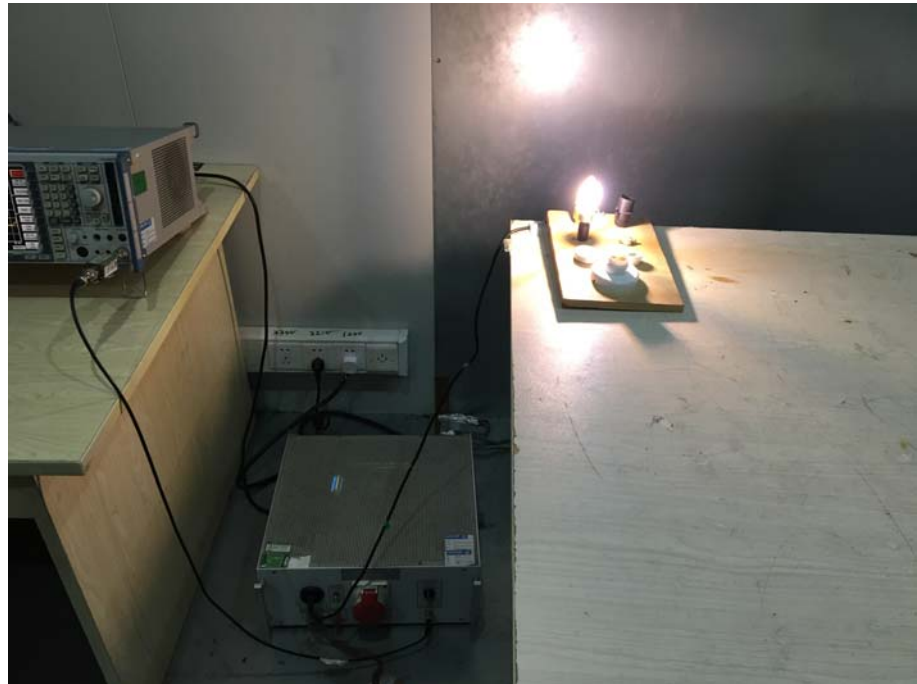
Conducted Emission Test Setup
