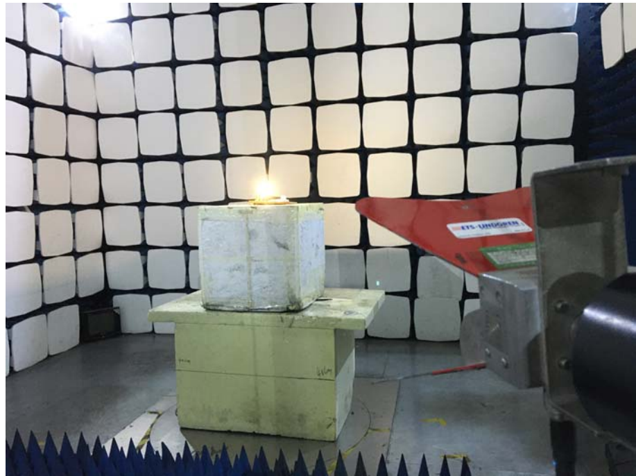
Radiation Emission Test Setup (1GHz to 18GHz)
