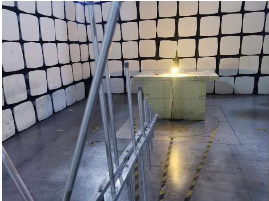
Radiation Emission Test Setup (30MHz to 1GHz)
