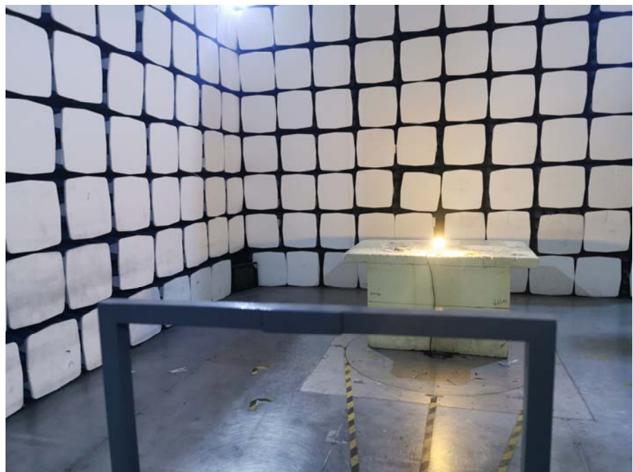
Radiation Emission Test Setup (Below 30MHz)
