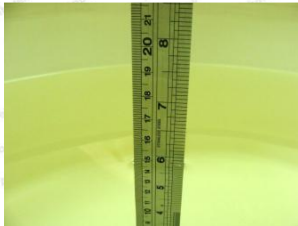
Photo of Liquid Height for Body SAR
