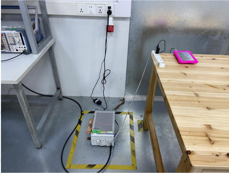
Photo of Power Line Conducted Emission Test
