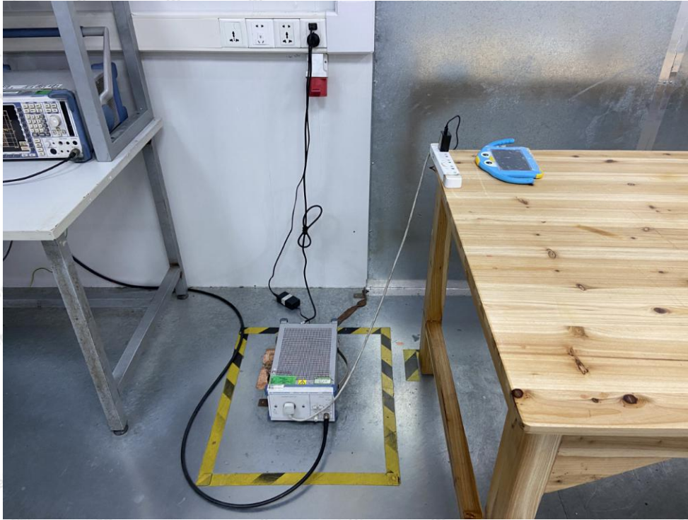
Photo of Conducted Emission Measurement
