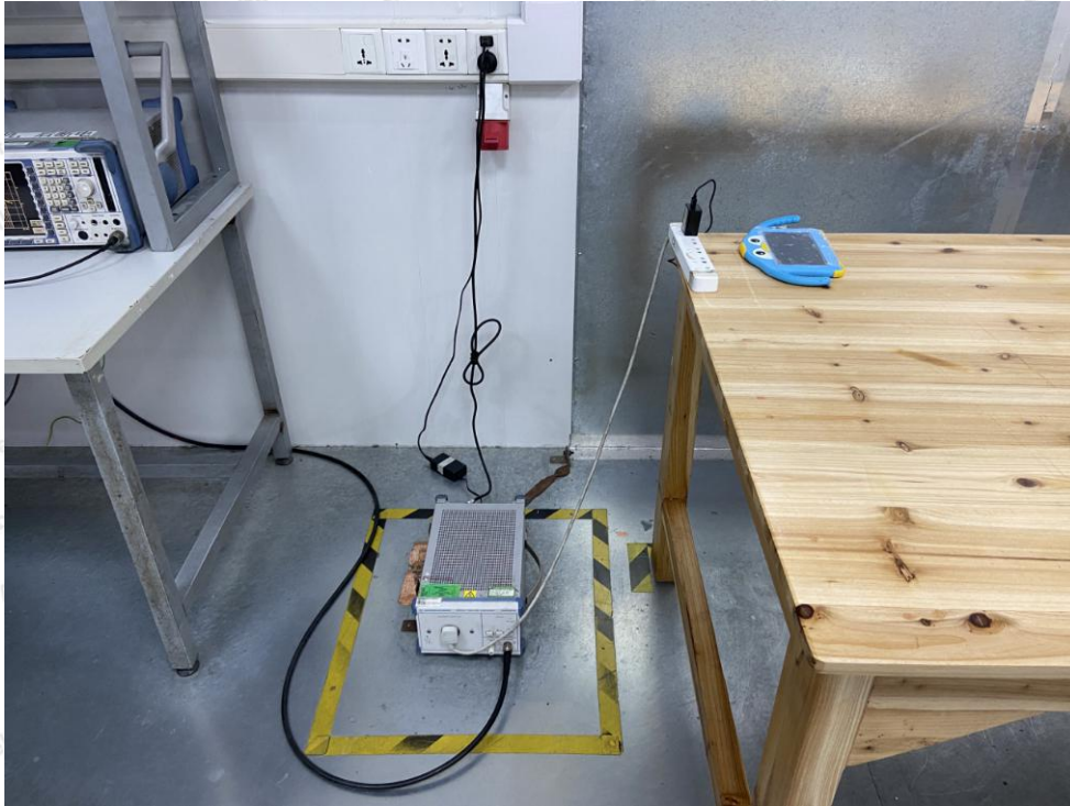
Photo of Conducted Emission Measurement
