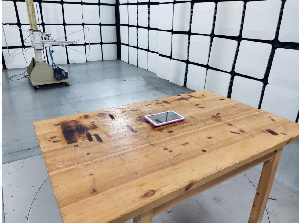
Photo of Radiation Emission Test
