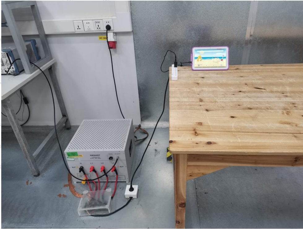
Photo of Conducted Emission Measurement
