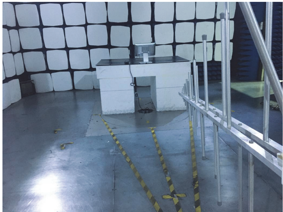
Radiation Emission Test Setup (30MHz to 1GHz)
