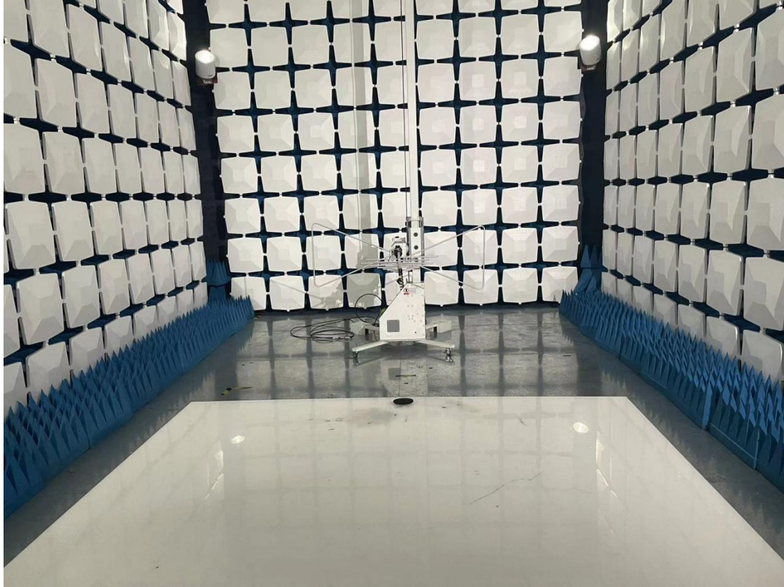
Blow 1GHz for radiated emission test setup
