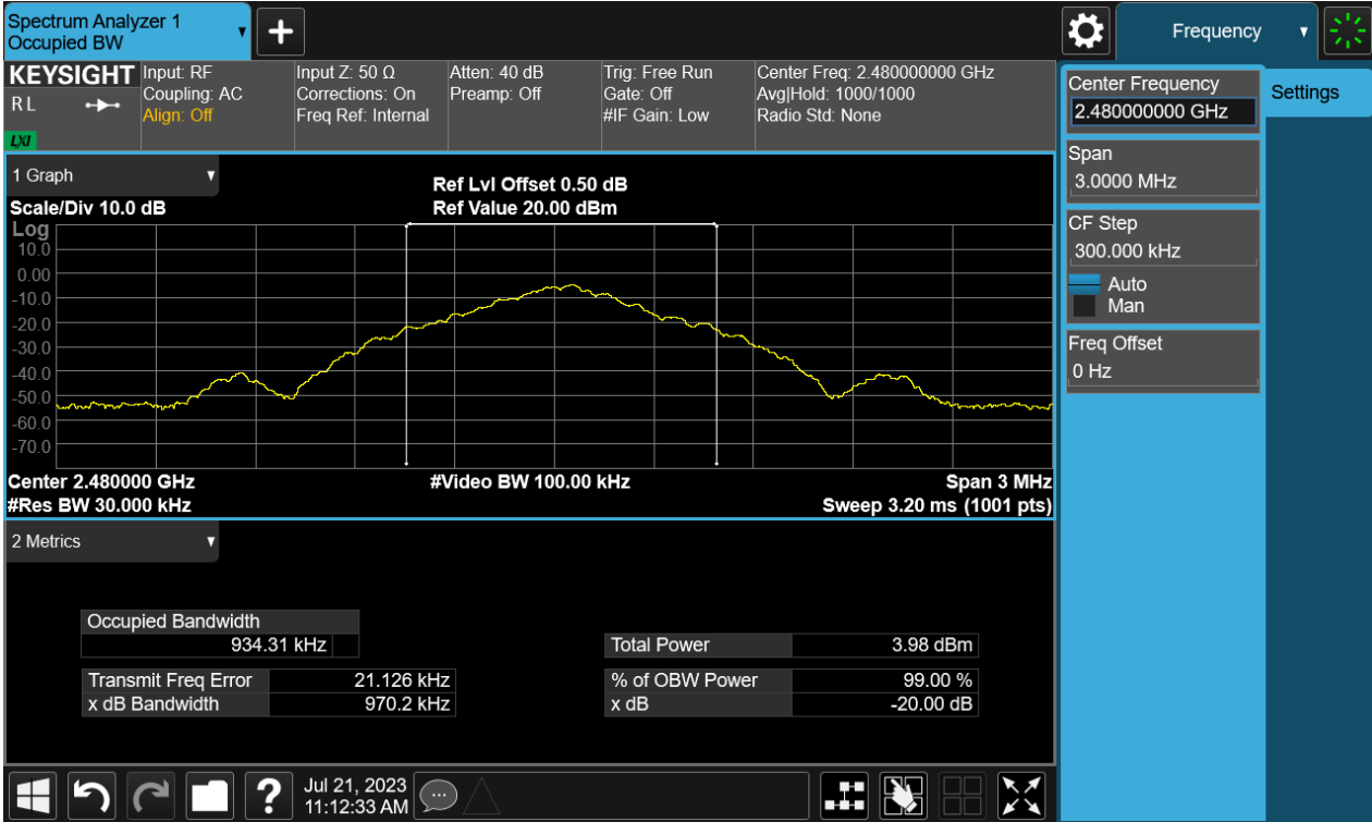
Figure 33: The plots of 20dB Bandwidth and 99% Bandwidth, 2480MHz
