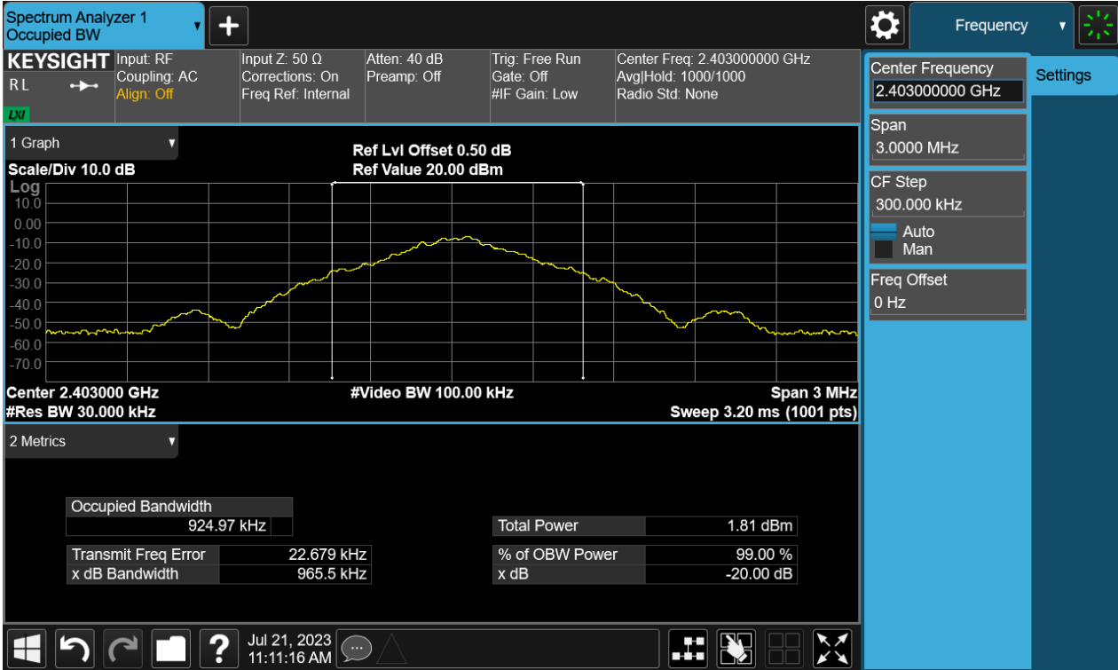
Figure 32: The plots of 20dB Bandwidth and 99% Bandwidth, 2442MHz
