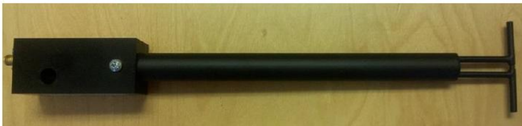
Figure 1 – MVG COMOSAR Validation Dipole
