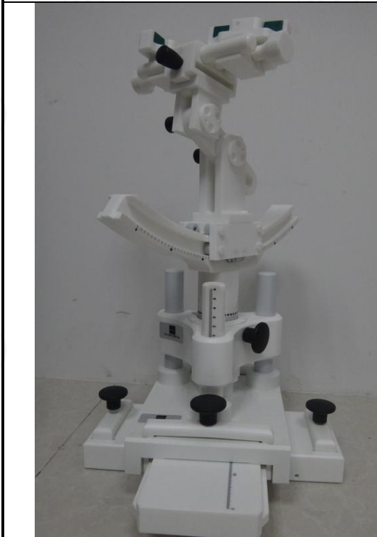
COMOSAR Mobile phone positioning system
