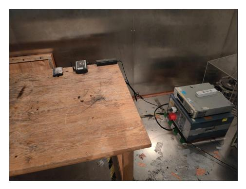
Radiated Emission below 1GHz test:
