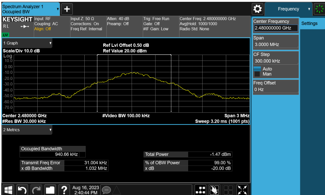
Figure 15: The plots of 20dB Bandwidth and 99% Bandwidth, 2480MHz
