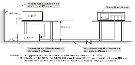
The setup of EUT is according with per ANSI C63.10-2013 measurement procedure. The specification used was with the FCC Part 15.207 and RSS-GEN limits.
