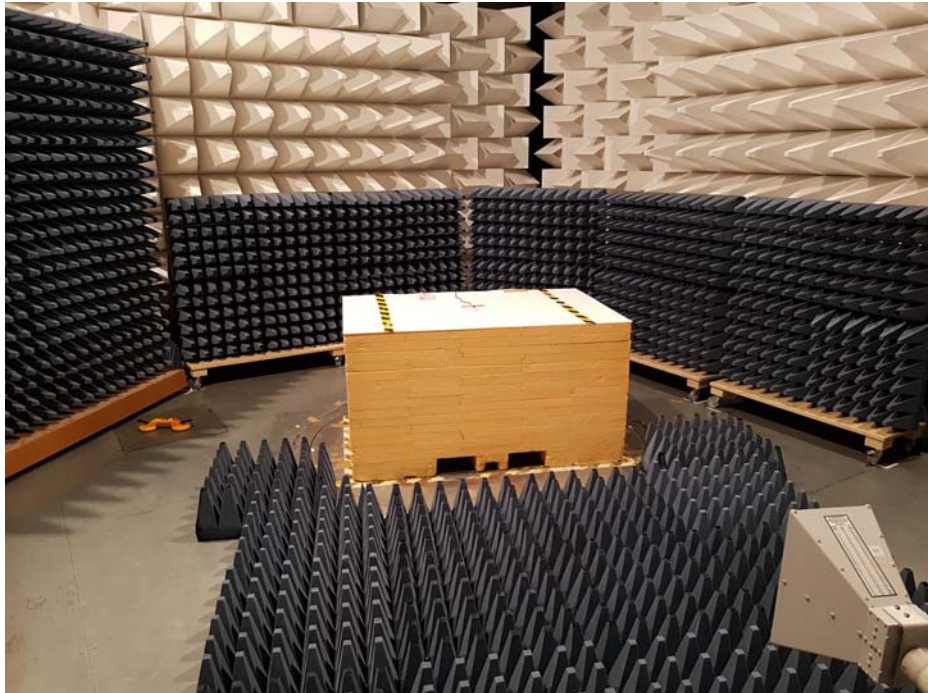
Figure 5 EUT / set up - test module ER2 (radiated emissions 1 - 18 GHz)
