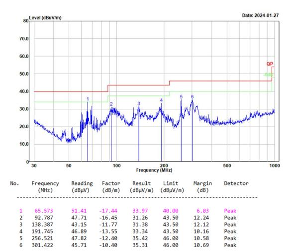
Project No.: CR240105113-RF Tester: Vic Du Polarization: vertical Note: Transmitting BLE
