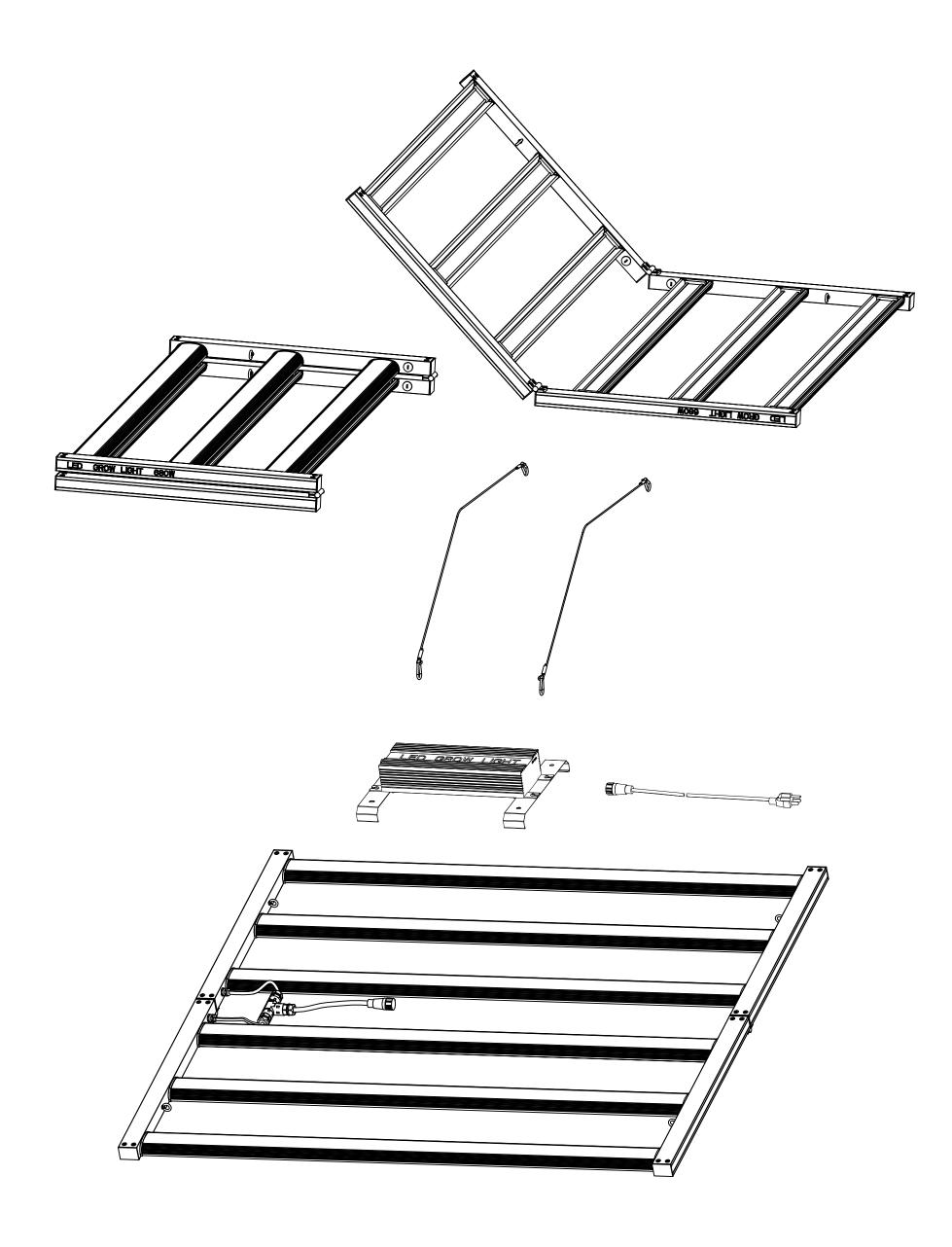
2 Position the drive power assembly on the back of the lamp body.
