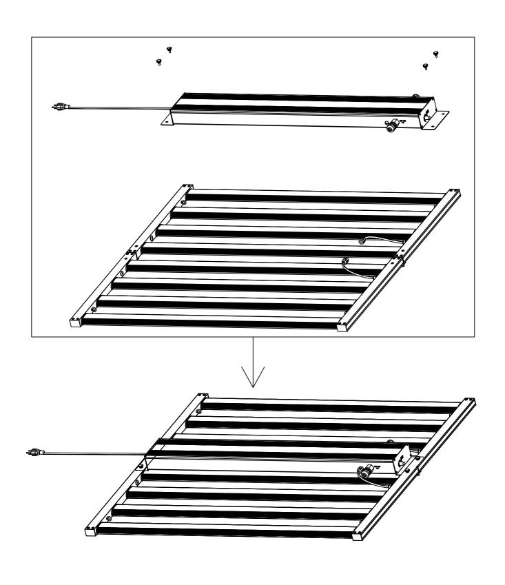
3 Wiring the drive power assembly.
