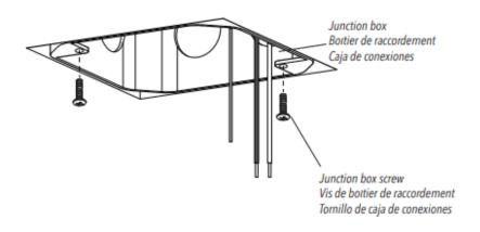
3. Connect the white wire (N) from the light fixture to the white supply wire (N) from the junction box using a wire connector. Connect the black wire (L) from the light fixture to the black supply wire (L) from the junction box using a wire connector. Connect the ground wire (G) from the light fixture to the ground supply wire (G) from the junction box using a wire
