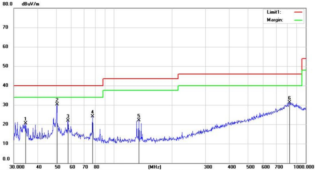
Site 3m Chamber #1 Polarization: Vertical Temperature: 22 C
