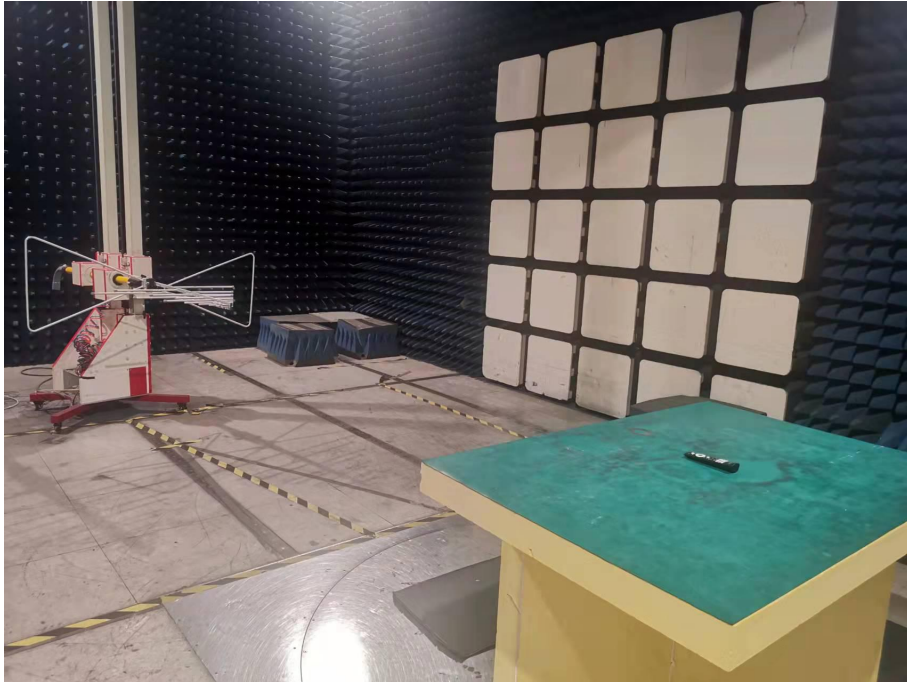
Spurious Emission Test Setup (30MHz-1GHz)
