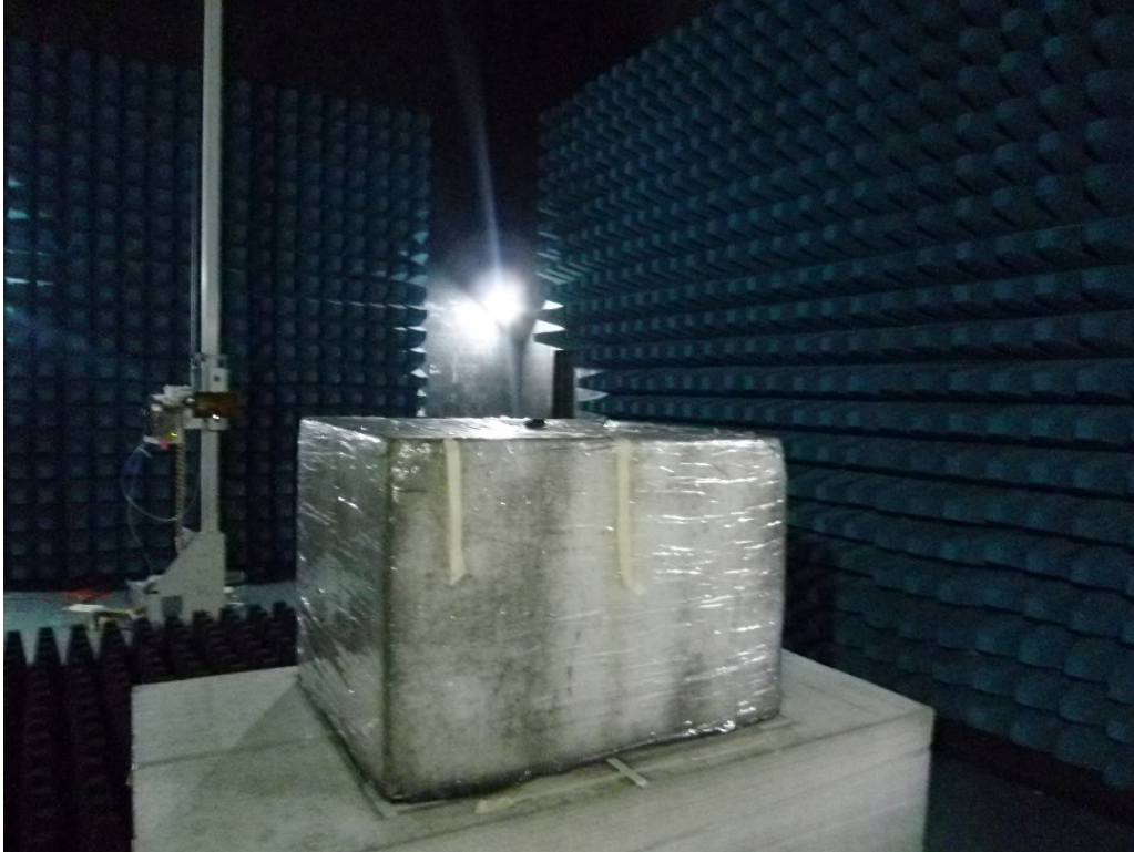
Radiated Emission Set up Photos (Front View)
