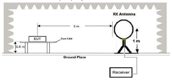
(2) Radiated Emission Test-Up Frequency 30MHz~1GHz
