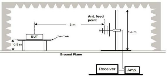
(3) Radiated Emission Test-Up Frequency Above 1GHz
