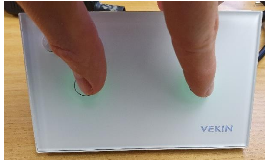
Figure 2: Holding down the two buttons (>10s)
