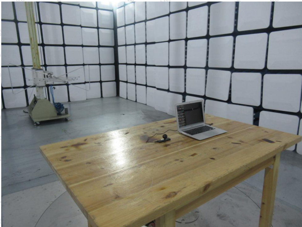
Photo of Radiation Emission Test
