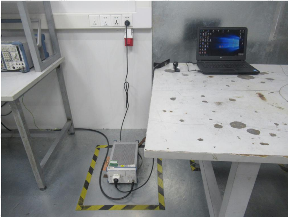
Photo of Conducted Emission Test
