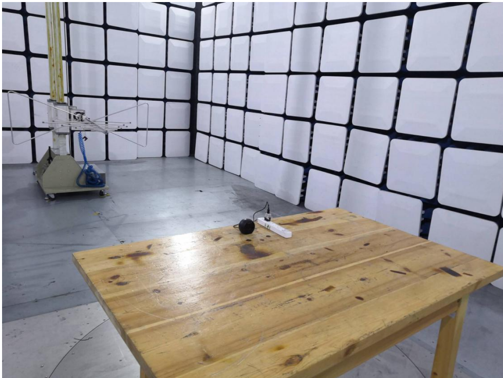
Photo of Radiation Emission Test
