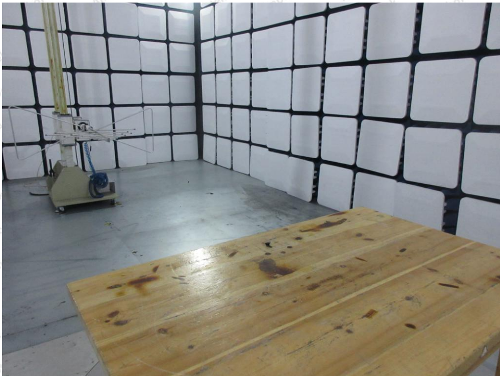
Photo of Radiation Emission Test
