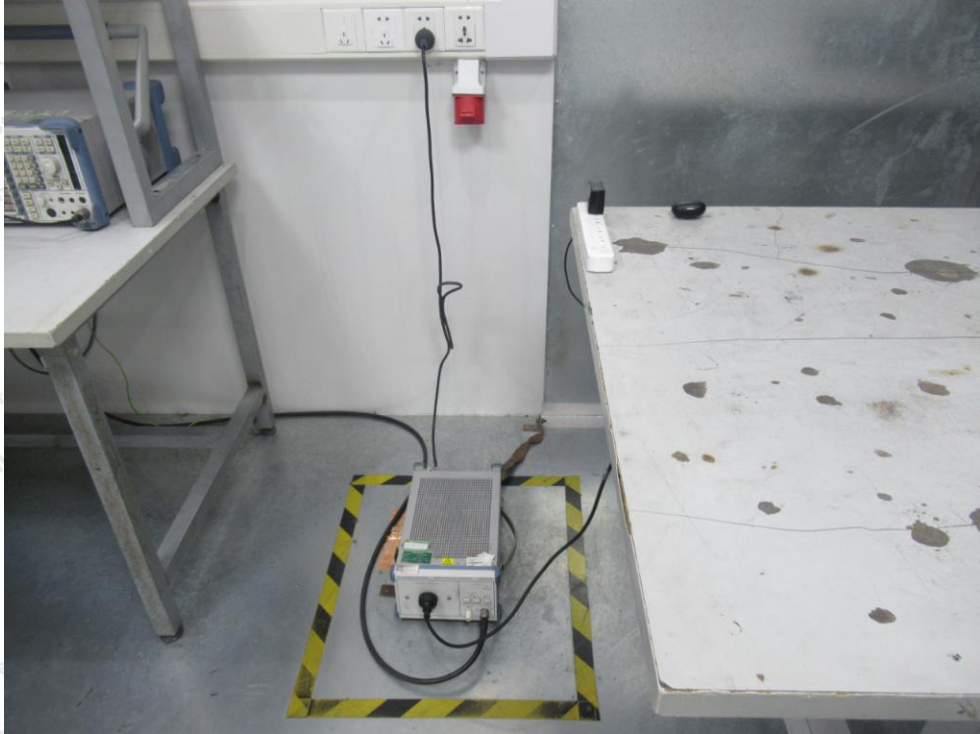
Photo of Conducted Emission Measurement
