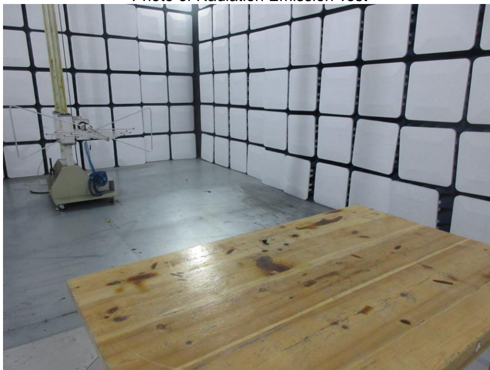
Photo of Radiation Emission Test
