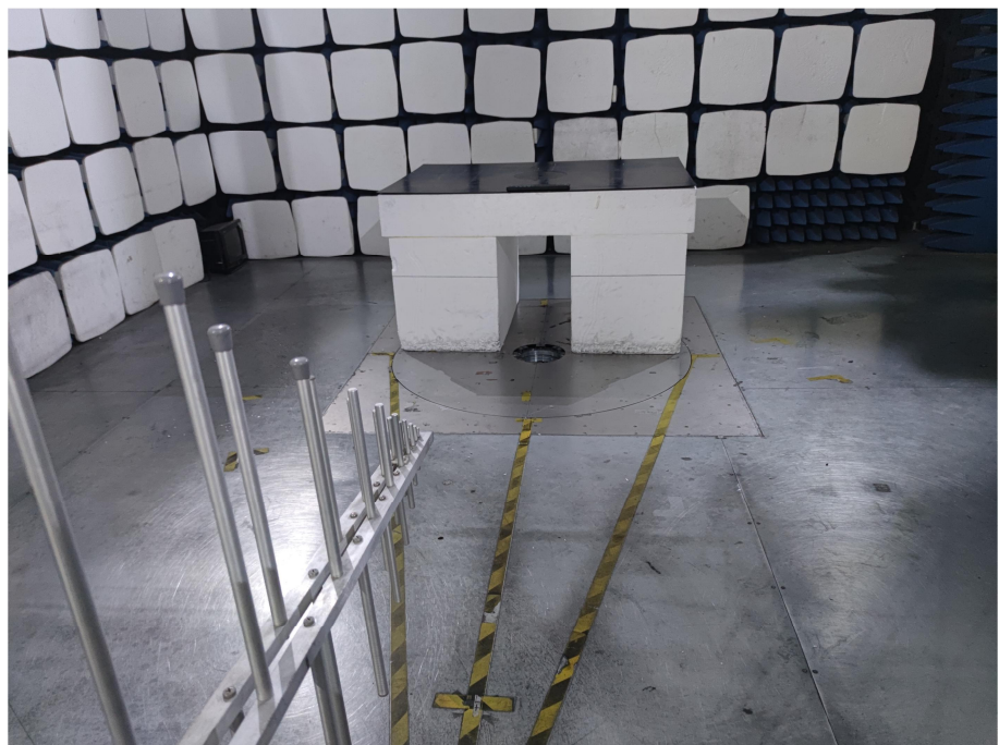
Radiation Emission Test Setup (30MHz to 1GHz)
