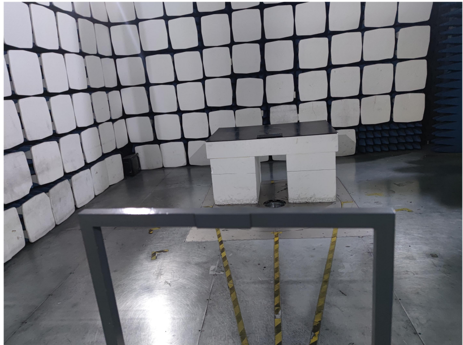
Radiation Emission Test Setup (Below 30MHz)
