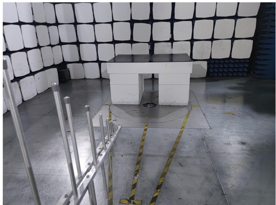
Radiation Emission Test Setup (30MHz to 1GHz)
