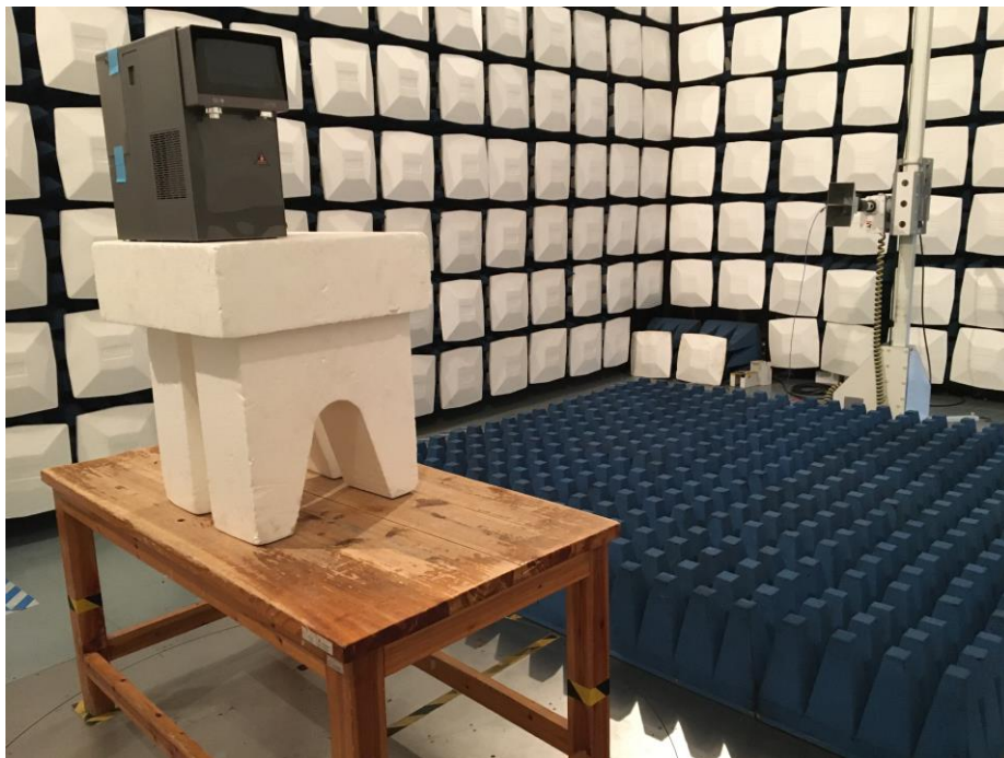
Test Setup For Radiated Emission (Above 1GHz)
